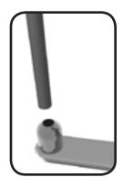
Insert pole into the chrome piece on the foot.
