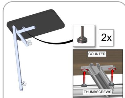
Install counter to mounting tube with 8/32" thumb screws, repeat for second screw.
