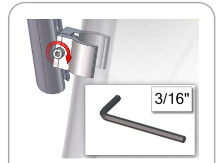
Secure second tube clamp TC-30 around backwall and tighten with 3/16" hex key tool.
