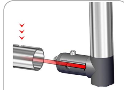
Use TC-30-90B to connect bottom frame corners; snap on button.
