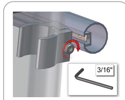
Secure tube clamp TC-30 around backwall at desired height and tighten with 3/16" hex key tool.
