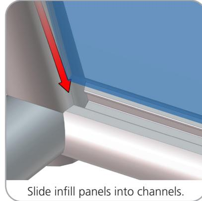
Slide infill panels into channels.
