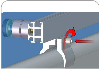
Using hex key turn bolt clockwise to tighten tube clamps, securing graphic header to backwall.
