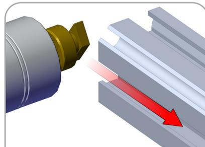
Before attaching to graphic, slide end of stand off (CKSO) into extrusion. Repeat for other stand-off(s).
