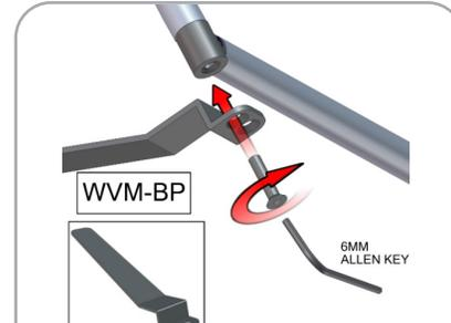
Using provided allen key, secure both feet (WVM-BP) to bottom of frame by tightening bolt.
