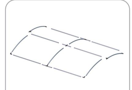
Frame assembly is complete once all sides and middle are connected.
