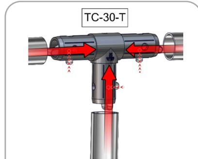
Connect sides of frame by lining up holes with snap buttons.
