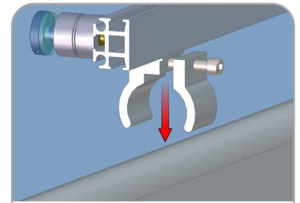
Once graphic is attached to stand-offs and extrusion, position tube clamps (TC-30) onto backwall.
