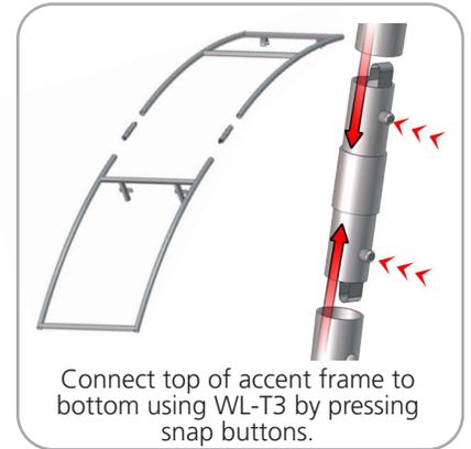
Connect top of accent frame to bottom using WL-T3 by pressing snap buttons.
