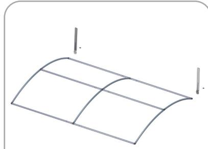
Attach feet with Allen key. See next step for detailed view.
