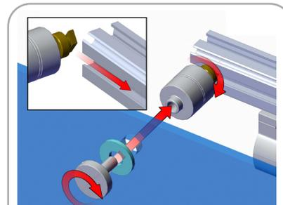
Attach graphic to stand-offs and extrusion with washer & other end of stand-off. Turn clockwise to secure.
