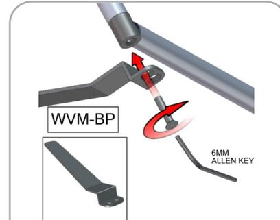
Using provided allen key, secure both feet (WVM-BP) to bottom of frame by tightening bolt.
