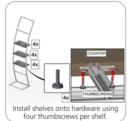
Install shelves onto hardware using four thumbscrews per shelf.
