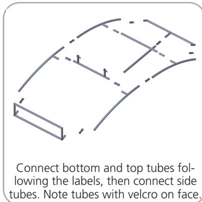
Connect bottom and top tubes following the labels, then connect side tubes. Note tubes with velcro on face.
