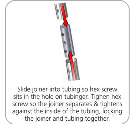
Slide jointer into tubing so hex screw sits in the hole on tubing. Tighten hex screw so the jointer separates & tightens against the inside of the tubing, locking the jointer and tubing together.
