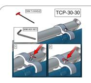
Using provided 5mm hex key, rotate bolt clockwise to secure accent to top of fabric backwall.
