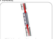
Slide joiner into tubing so hex screw sits in the hole on tubinger. Tighen hex screw so the joiner separates & tightens against the inside of the tubing, locking the joiner and tubing together.
