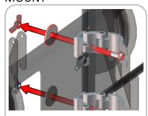
Attach ACC60 clamps to monitor mount with a bolt and washer, tighten with wingnut.
