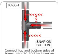
Connect top and bottom sides of frame using TC-30-T by lining up holes with snap buttons.
