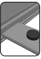
Center the foot, tighten the knob. Assemble bungee pole.
