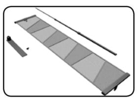
Remove the system from outer packaging and carry bag. Insert foot into notch in on bottom rail.
