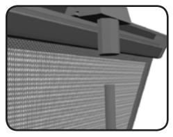
Place the rail on the top pole, with the pole inside the hole in the plastic protrusion
