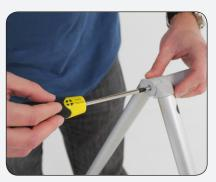
**Step 3** Repeat steps 1 and 2 for second 3 piece pole section. These 3 piece poles will make the width of the frame.
