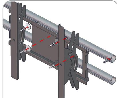
Secure monitor mount with washers and wingnuts.
