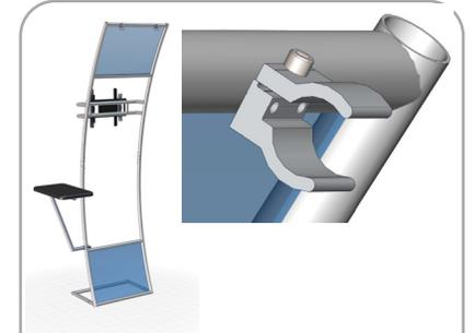
Tube clamps will come attached to frame. Position accent in front of backwall in desired location.
