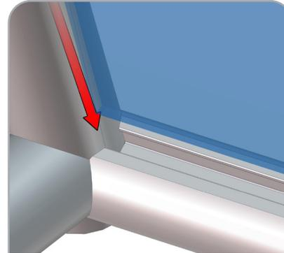
Slide infill panels into channels.
