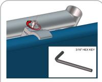
Using provided 3/16" hex key, rotate bolt clockwise to secure accent to top of fabric backwall.
