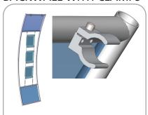
Tube clamps will come attached to frame. Position accent in front of backwall in desired location.
