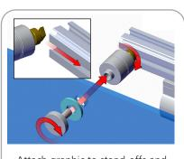
Attach graphic to stand-offs and extrusion with washer & other end of stand-off. Turn clockwise to secure.
