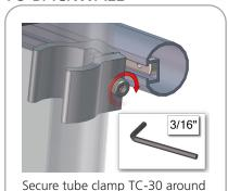
Secure tube clamp TC-30 around backwall at desired height and tighten with 3/16" hex key tool.
