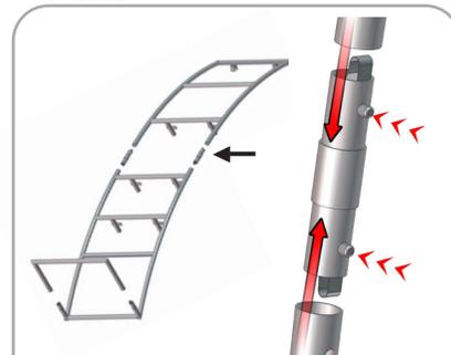
Connect top of accent frame to bottom using WL-T3 by pressing snap buttons.
