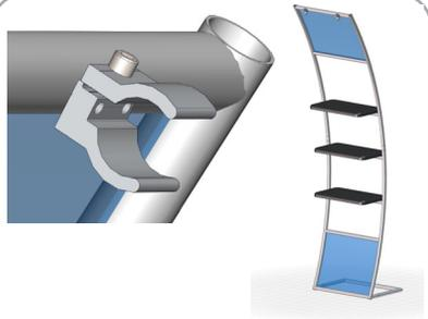
Tube clamps will come attached to frame. Position accent in front of backwall in desired location.
