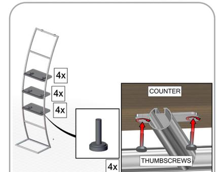
Install shelves onto hardware using four thumbscrews per shelf.
