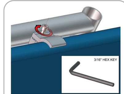
Using provided 3/16" hex key, rotate bolt clockwise to secure accent to top of fabric backwall.
