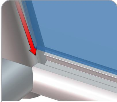
Slide infill panels into channels.
