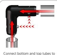
connect bottom and top tubes to side tubes following the labels.
