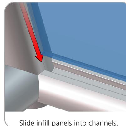
Slide infill panels into channels.
