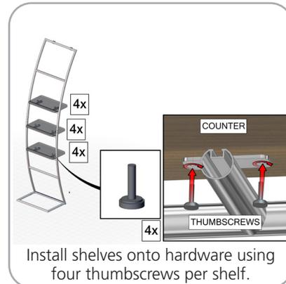
Install shelves onto hardware using four thumbscrews per shelf.
