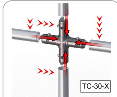
Use TC-30-X to connect middle frame sections; snap on button.
