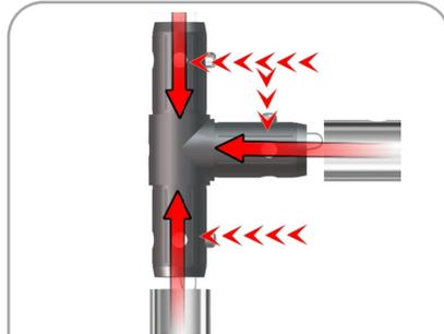
Connect top and bottom sides of frame using TC-30-T by lining up holes with snap buttons.
