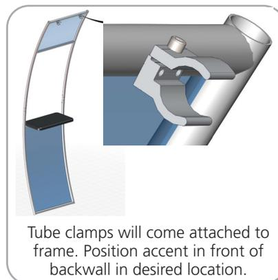
Tube clamps will come attached to frame. Position accent in front of backwall in desired location.
