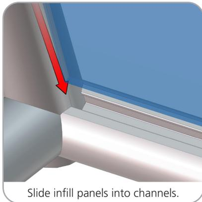
Slide infill panels into channels.
