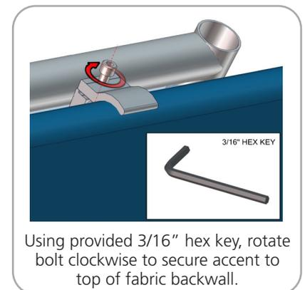
Using provided 3/16" hex key, rotate bolt clockwise to secure accent to top of fabric backwall.
