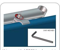
Using provided 3/16" hex key, rotate bolt clockwise to secure accent to top of fabric backwall.
