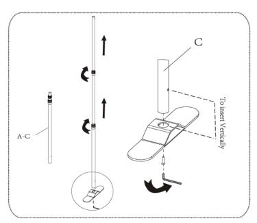
To insert pole #A-C into the socket of base vertically then tightening; Afterwards, screw off #A-C to the limited stop and screw up the plastic bolt.
